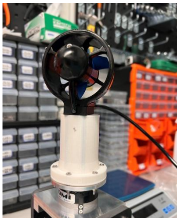
Figure 2.3. Direct coupling relationship between thrusters and sensors
